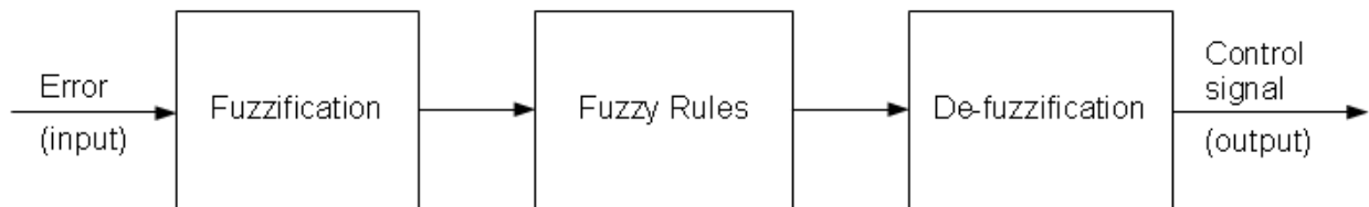
Fig 25 Fuzzy Logic Controller Topology
