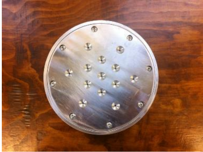
Figure 4-13 The bottom plate of air bearing device made in workshop
