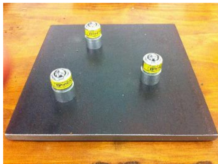
Figure 3-17 Beneath view of ball-bearing pallet
