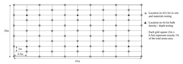
Figure 1. Sample locations used to assess spatial analysis using in-situ and laboratory materials testing (n=61) for an equestrian arena surface.
