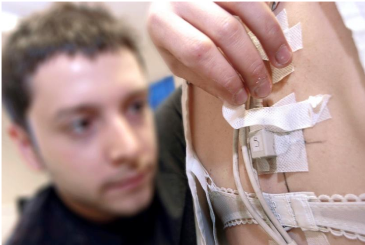
Figure 45 Fixation of the sensors (sensors fixed to HypaFix tape with double-sided tape, reinforce with additional HypaFix tape on side and top. Drinking straws used for cable management and to reduce the effect of the weight of the cables on sensors)
