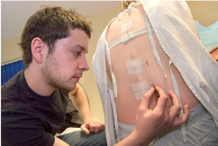
Figure 44 Fixation of the sensors: use of protective HypaFix tape
