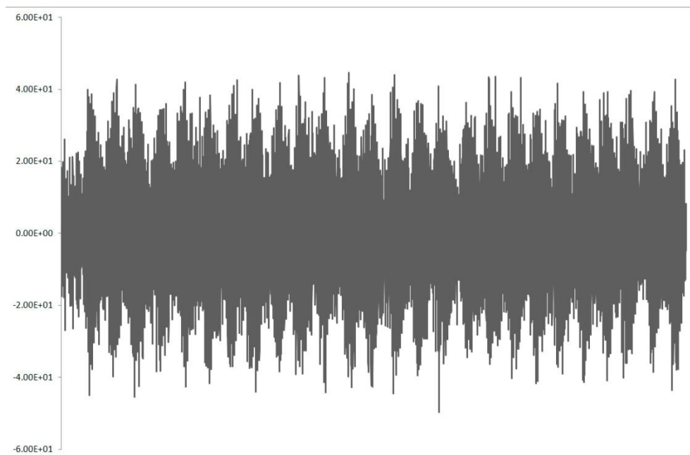
Figure B-1-3 T8 raw data high-pass filtered at 10 Hz
