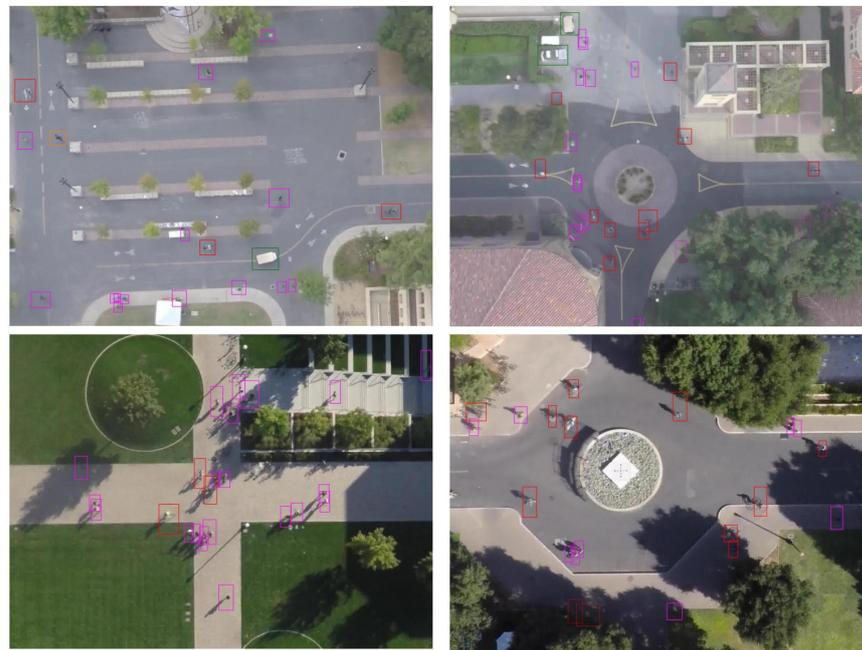
**Figure 1.** Objects in UAV images are usually small in size (proportional to total image size) and general purpose object detectors are not designed to cope with it [11].
