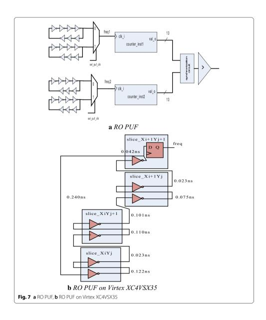
bit binary counters and a crossing clock domain circuit are necessary in order to compute one RO PUF answer. The cryptographic key used with Salsa 20/20 involves 128 PUF circuits.
