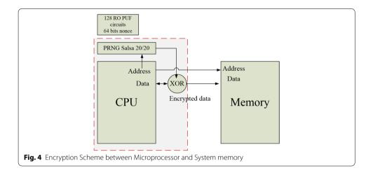
core (marked with dotted line in Fig. 3). The authentication relies on knowing the same pseudorandom key. If two IP cores are allowed to exchange data, their wrappers will generate the same pseudorandom sequences. The microprocessor from one domain may read a mixed bit value of a pseudorandom key and compare it with its one mixed bit value. Confirming the identity of the data source contributes, along the encryption/decryption operations, to counteract the security threats presented in Sect. 2.
