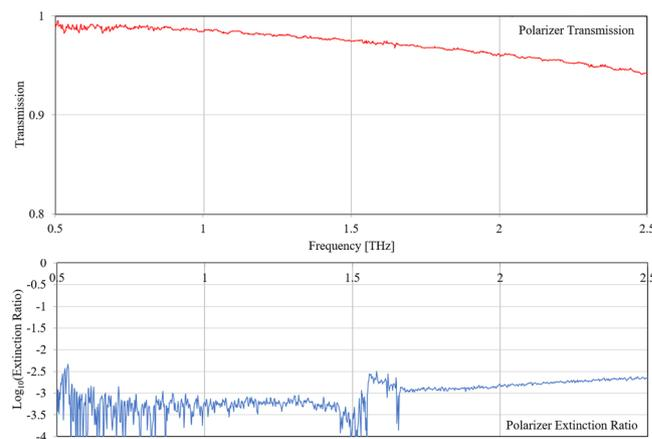
**Figure 3.** Top: Spectral Transmission of an identical photo-lithographic broadband polarizer to the one initially used in the system. Bottom: Extinction ratio of the same polarizer for the orthogonal polarization. This shows a transmission higher than 95% for frequencies above 2 THz and an overall rejection of the orthogonal mode lower than 1%.
