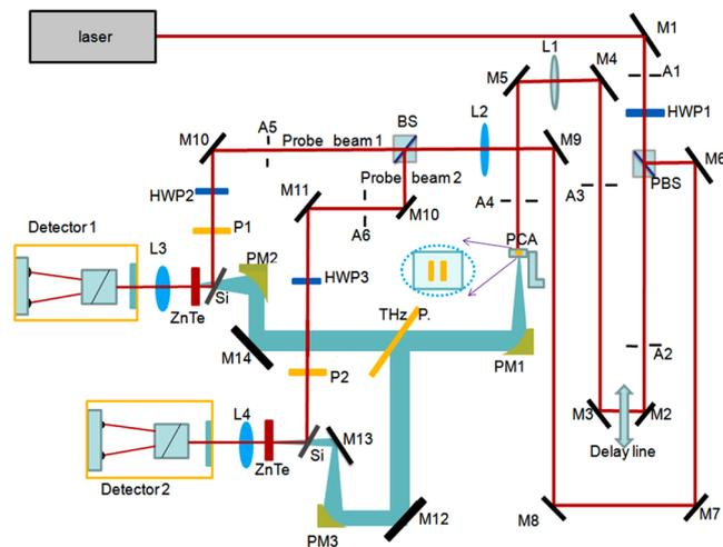
**Figure 1.** The overall system layout is shown with flat mirrors (M), optical lenses (L), off-axis parabolic mirrors for the THz beam (PM), iris apertures (A), half-wave plates (HWP) and polarizers (P). The THz polarizer is indicated with “THz P”. The PCA orientation is also shown providing horizontally polarized radiation. The two Silicon plates (Si) are also shown for THz/laser overlap and ZnTe crystals with the two detector units (with QWP + Wollaston prism) on the left.
