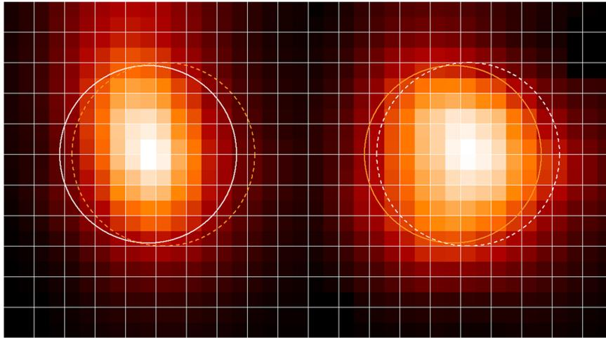
**Figure 8.** Amplitude maps of IG peak recorded in raster-scan mode. The rings show the cylinder envelope at which one sigma levels of power are contained (white in the beam and orange in the other for comparison).
