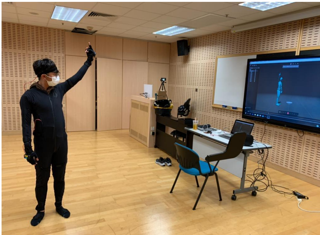
Figure 2. Calibrating the posture with the motion capture smartsuit
