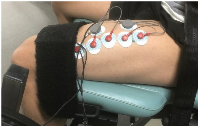
Figure 27. Three channel EMG array. Whole vastus lateralis muscle measured during 5-repetitions at three different speeds. This was conducted at Anglia Ruskin University, Cambridge. Position was determined using the same method as the NIRS (Seniam, 2020).
