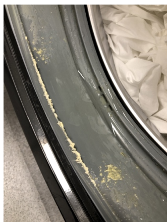
Figure 3 Typical image of drum seal residues after 100% paraffin-based ointment wash experiment at 30°C.
