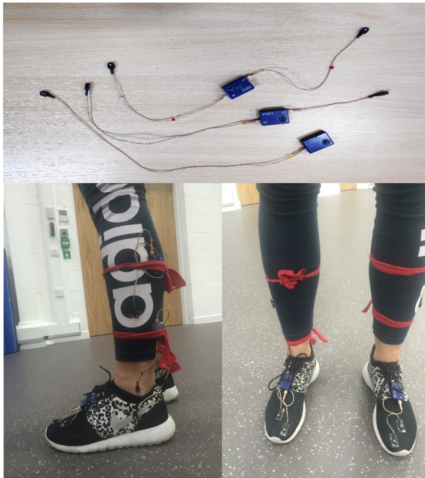
Figure 3.15. The markers were attached to participants' feet using double sided tape. To ensure the power does not become loose during the walking trials, they were tied with red elastic bands.
