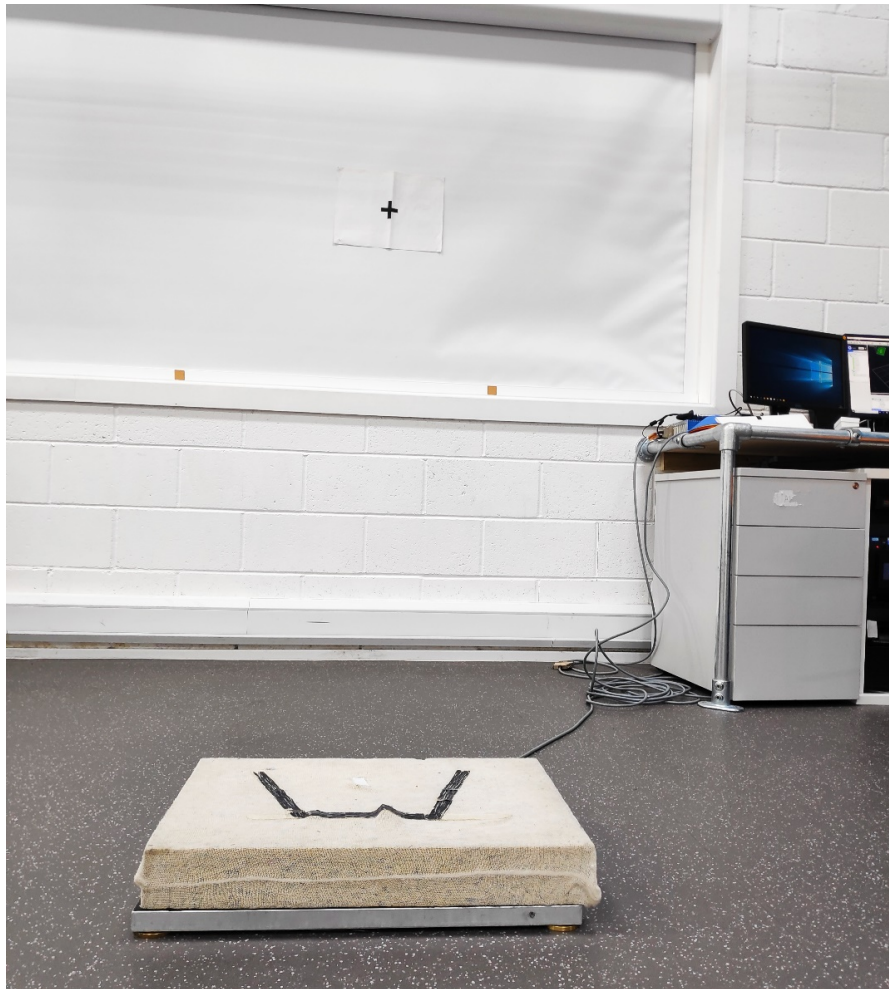
Figure 3.12. The compliant foam used to disturb the somatosensory system of the participants. The target used is also demonstrated, which was placed at eye level height of individuals. Those who could not see the target (SSI), were instructed to look straight ahead.
