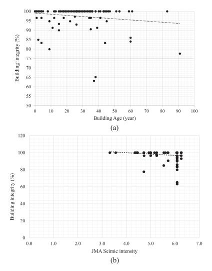
**Figure 1.** Impact of age and seismic intensity on building integrity ( $S_{cb}$ ). (a) Age. (b) JMA seismic intensity.
