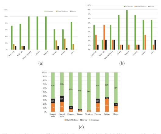
Figure 2. Building integrity. (a) Post-1981 building integrity. (b) Pre-1981 building integrity. (c) Loss of integrity distribution.
