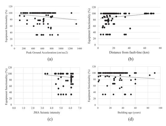
**Figure 9.** Influence of earthquake metrics and building age on equipment functionality. (a) Ground motion. (b) Distance. (c) Seismic intensity. (d) Building age.
