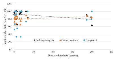
Figure 11. Building, critical systems, and equipment functionalities effect on evacuation.
