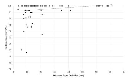
Figure 4. Impact of distance on building integrity.
