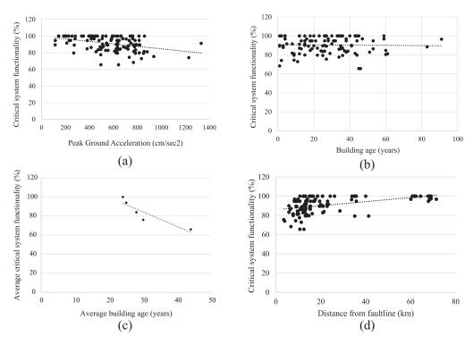
**Figure 6.** Influence of earthquake metrics and building age on the functionality of critical systems. (a) PGA. (b) Building age. (c) Average loss of functionality and average age. (d) Distance from fault line.
