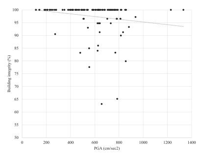
Figure 3. Effect of PGA on building integrity.
