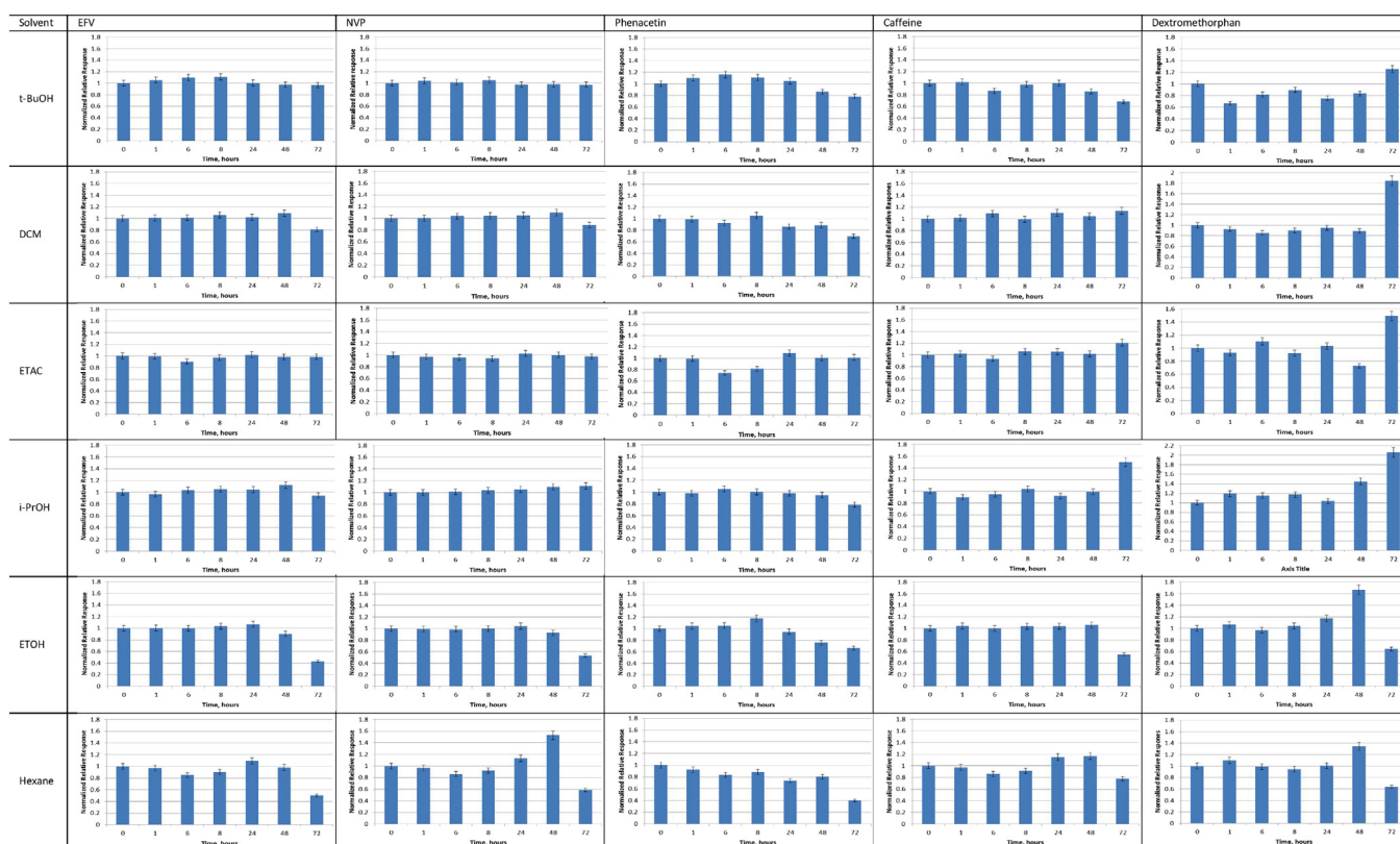
Fig. 5. Plot of normalized average response ratio vs time for EFV, NVP Phenacetin, Caffeine and Dextromethorphan for simulated street nyaope samples extracted with tertiary butyl alcohol, dichloromethane, ethyl acetate, isopropanol, ethanol and hexane respectively.
