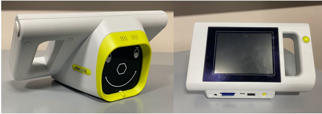
Figure 2.01: Left: Patient facing aspect of the PlusoptiX A12C auto-refractor, Right: Examiner facing aspect of the PlusoptiX A12C auto-refractor.
