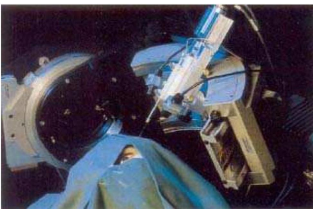
FIGURE 2 Ocular Robotic Prototype (ORP) with a drug delivery injector head and glass pipette. 43
